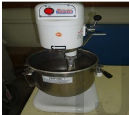
Figure 1: Paste / Mortar Mixer
